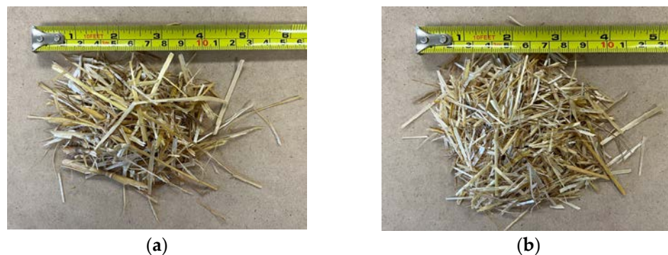
Figure 4. (a) 1 pass of the material, (b) 2 passes of the material. Source: Matías Soto Acuña.
