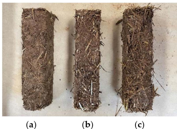
Figure 5. Samples (a–c) of clay plaster with their respective proportions.
